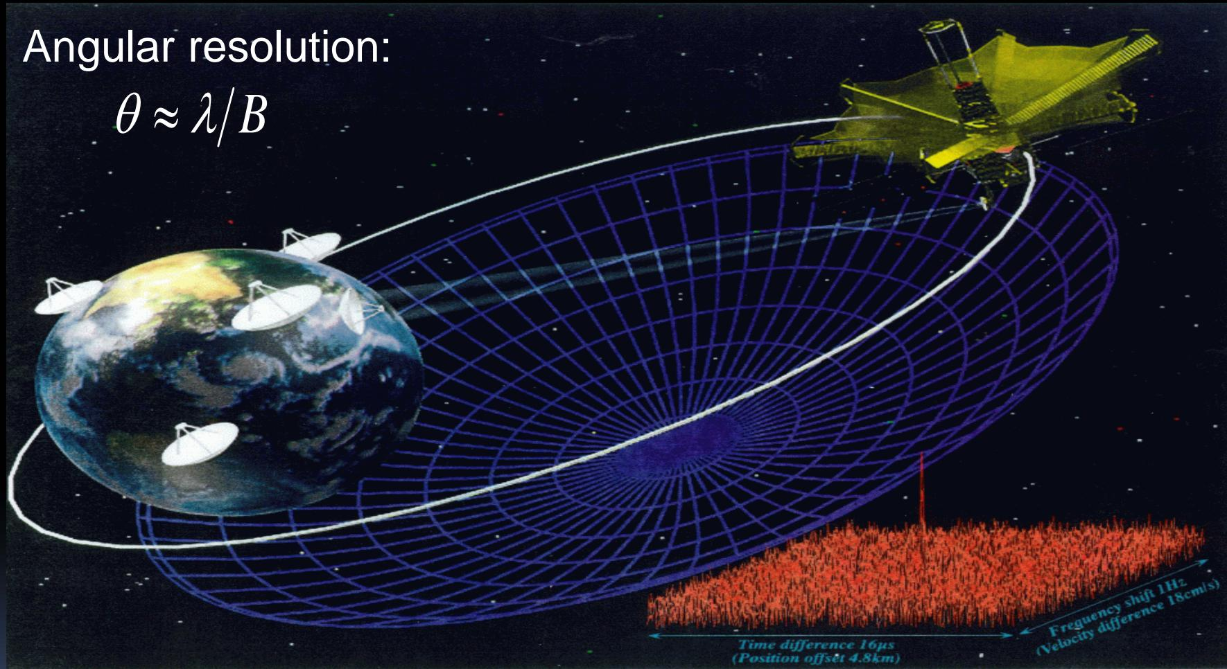
Ground-based VLBI:  $\lambda = 6 \text{ cm}; B = 10000 \text{ km} \Rightarrow \theta \approx 1.5 \text{ mas}$
