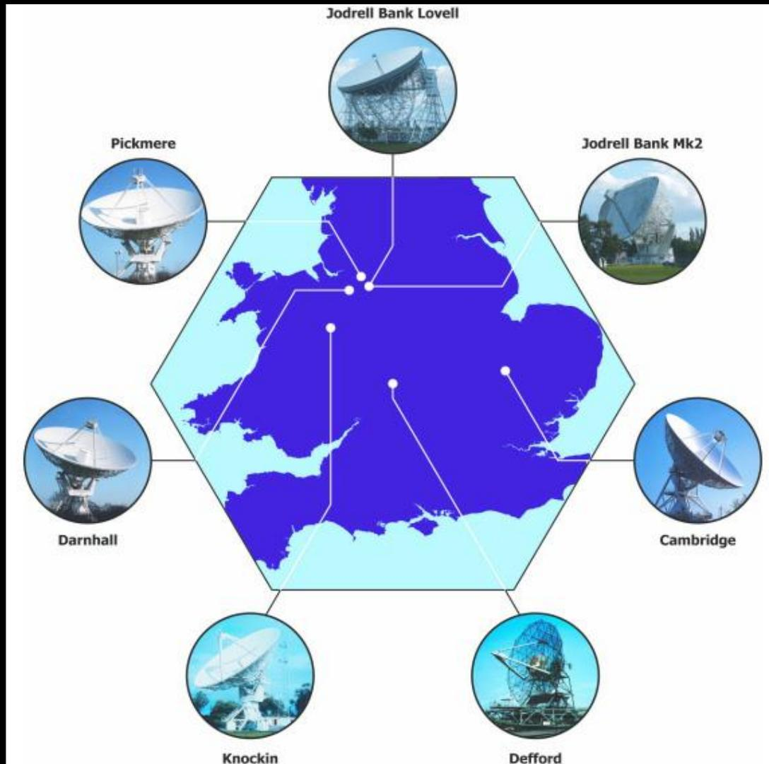
Multi-Element Radio-Linked Interferometer (MERLIN)
