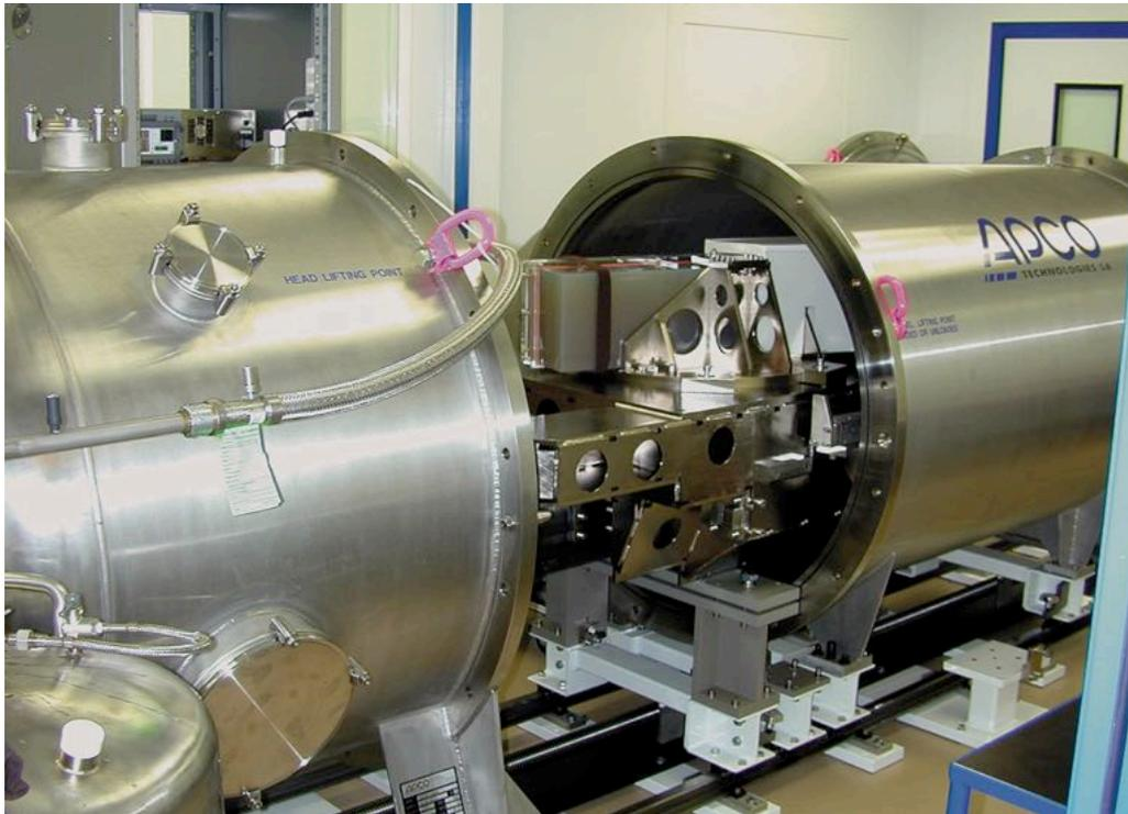
Spectrograph on a rigid bench, which is housed in a vacuum tank.
