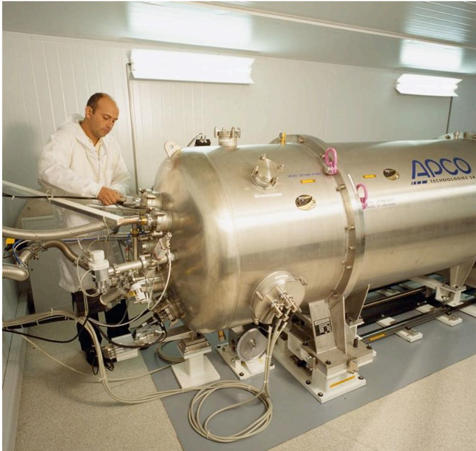
Spectrograph on a rigid bench, which is housed in a vacuum tank.
