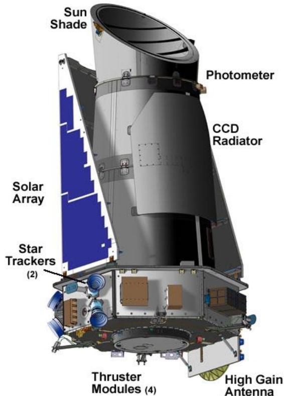
A custom-built, 0.95m diameter space telescope dedicated to finding transiting planets
