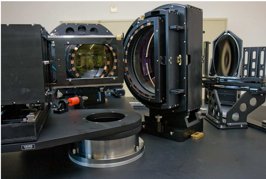
Figure 11. The SIFS – SOAR Integral Field Unit Spectrograph, the first spectrograph built by Brazilian astronomers. (© B. Barbuy)
