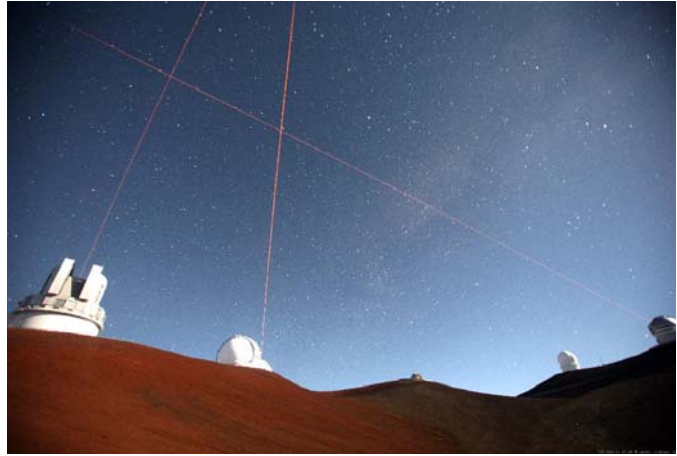
Figure 1 – Laser AO operations on Mauna Kea are arguably the most advanced on any site worldwide, as demonstrated here with sodium lasers being concurrently propagated by Keck, Subaru, and Gemini. The considerable experience Gemini is gaining from the ALTAIR LGS system is being incorporated into MCAO at Gemini-S. Photo credit: Subaru Observatory
