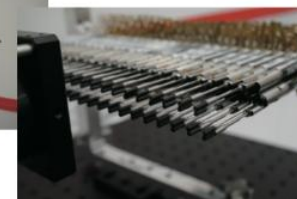
Fiber positioner "Cobra"
