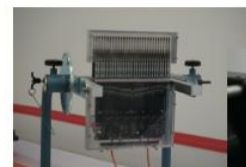
Fiber positioner "Cobra"
