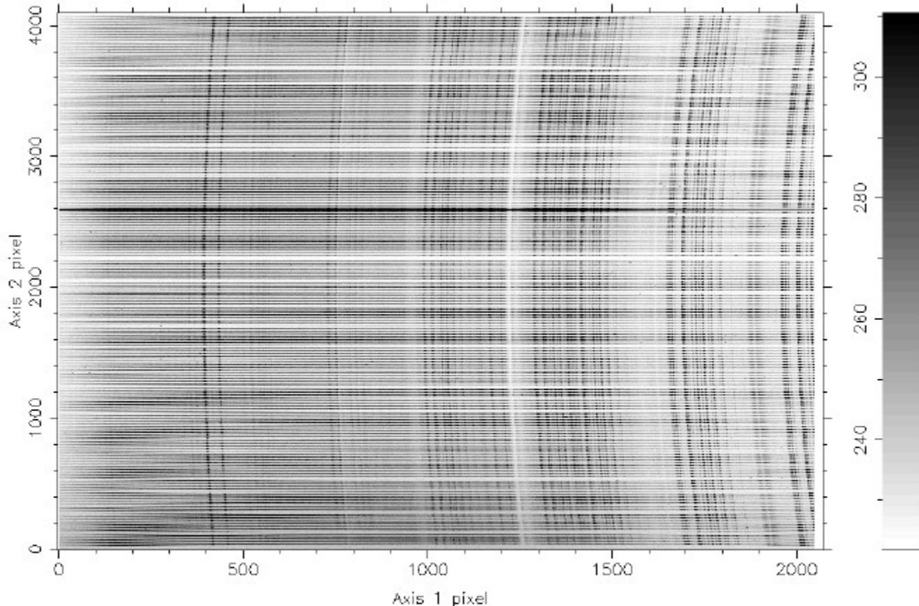
**Figure 3.** This 2hour ( $4 \times 1800$ sec) raw AAOmega frame shows the full 2D CCD frame containing the 392 science fibre spectra. Dispersion runs left to right in the low resolution red ( $\lambda_{\text{cen}}=7250\text{\AA}$ ,  $R \sim 1300$ ) unextracted spectra. Note the spectral curvature in the unsubtracted sky emission lines.
