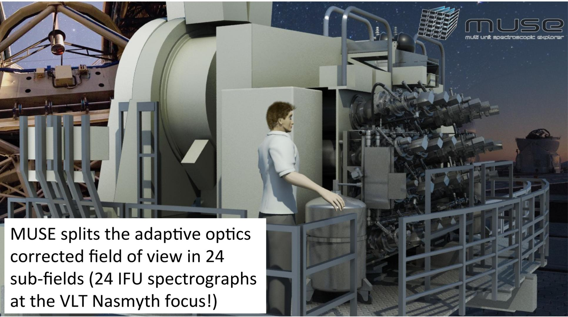
MUSE splits the adaptive optics corrected field of view in 24 sub-fields (24 IFU spectrographs at the VLT Nasmyth focus!)
