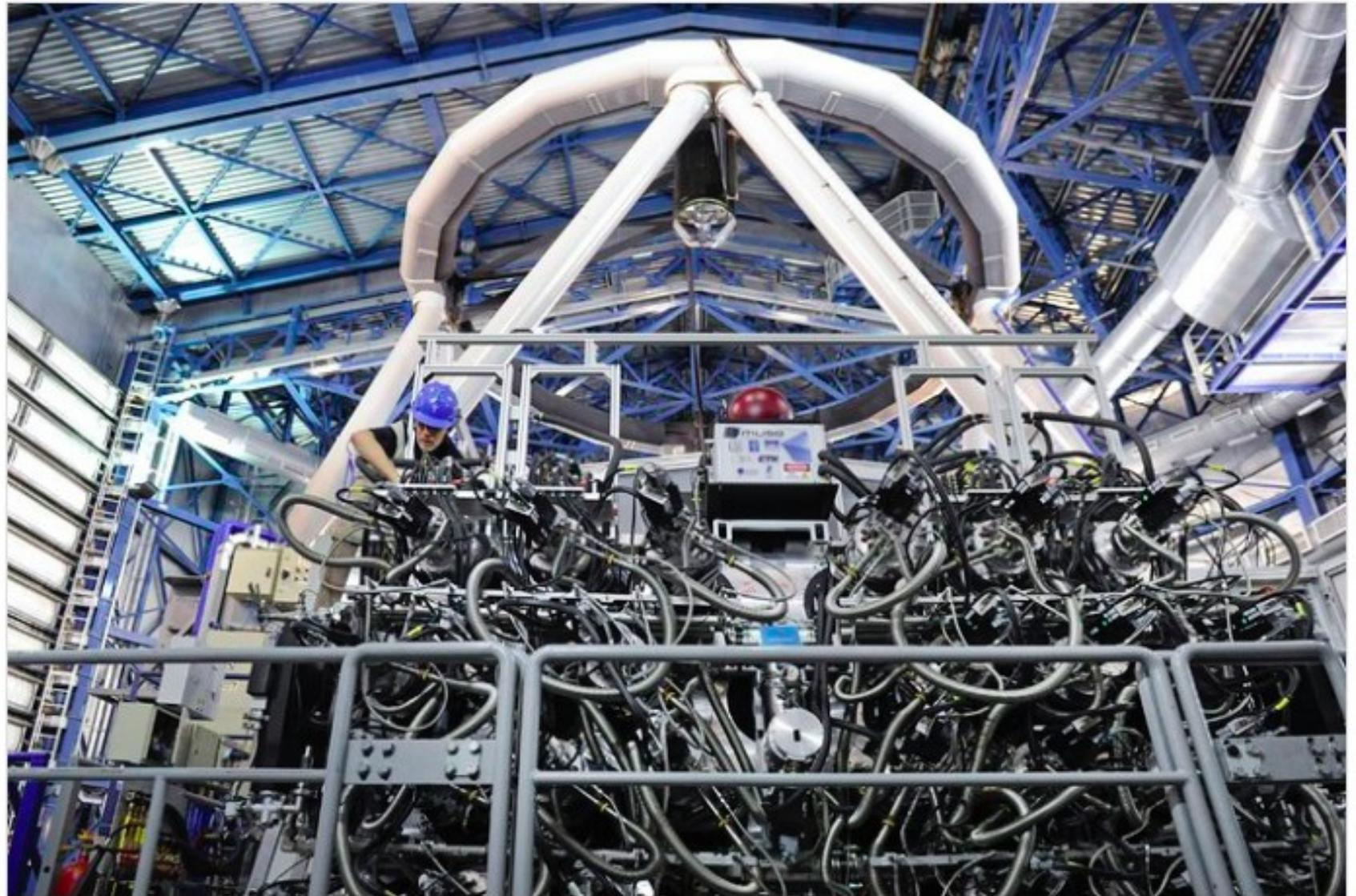
The MUSE instrument is one of the most recent additions to the instrument complement of the VLT. It has 24 detectors, each of which needs its own continuous flow cooling systems. Such innovative systems were first developed at ESO for the
