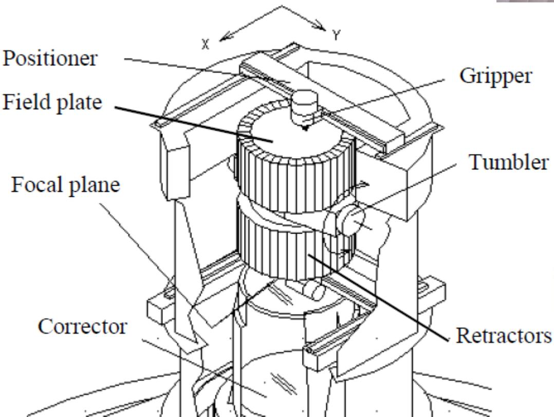
Figure 2 Cutaway view of 2dF positioner and plate exchanger
