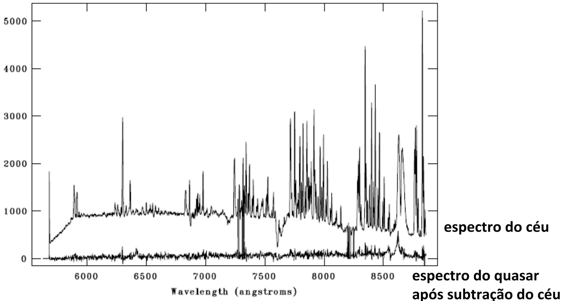
Figure 4. An example spectrum shows the  $\sim 1\%$  sky subtraction which can be routinely achieved with AAOmega. The lower trace shows the spectrum of the underlying faint quasar target once the strong night sky spectrum (upper trace) has been subtracted. Bad pixel masking has not yet been full integrated into the reduction software, as evidenced by the two
