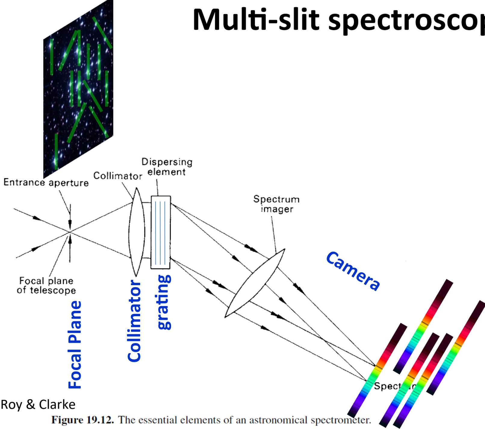
Figure 19.12. The essential elements of an astronomical spectrometer.
