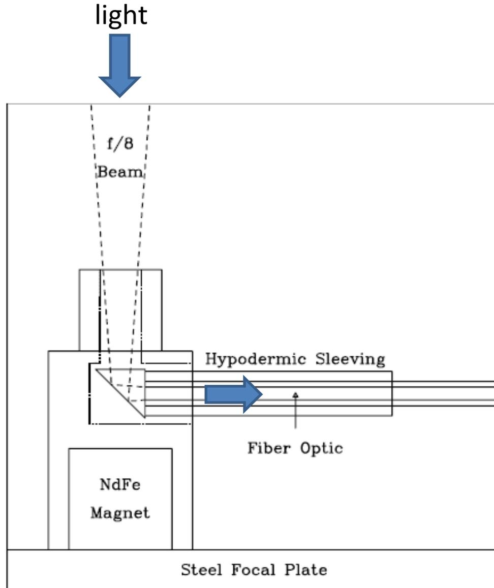
Figure 1: Schematic view of a fiber button on the focal plate.
