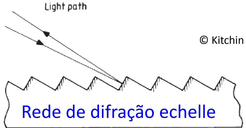
Figure 4.1.7. Enlarged view of an echelle grating.
