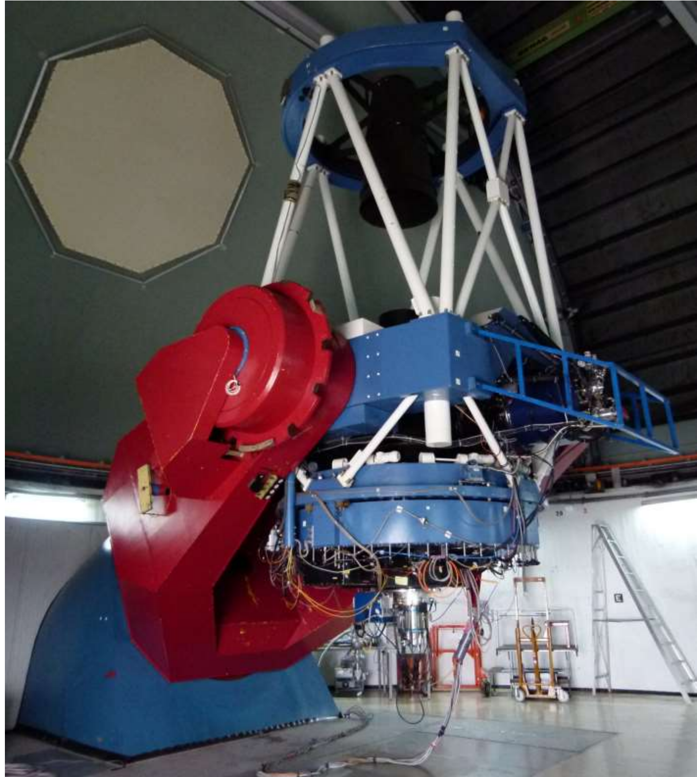
2,2 m telescope at La Silla Fork mount
