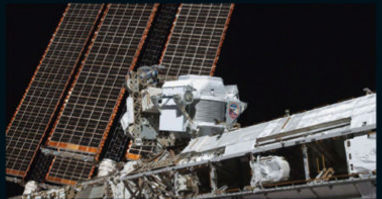
Reaching a sensitivity that allows the instrument to test a greater volume of the universe than its predecessor for primordial antimatter, the AMS will study the composition of cosmic rays with a high accuracy for a decade from the ISS
