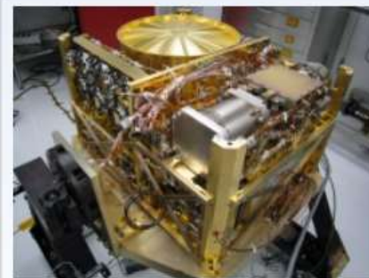
The Sample Analysis at Mars instrument suite, prior to its installation on the Curiosity rover.
