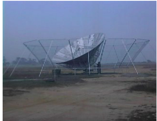
The GEM experiment (5.5 m fast spinning antenna)
