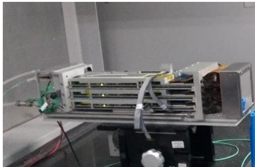
Detector Backend – Local HPC for on-flight tomography data processing and rendering
