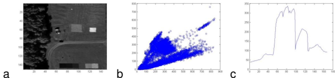
Mean of the data cube (a), scatterplot of the data cube for wavelengths number 60 and 120 (b), and mean spectrum (c)
