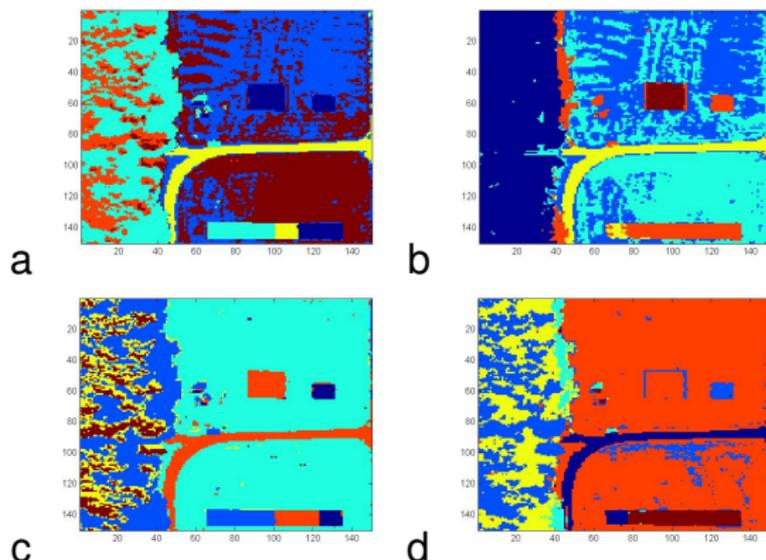
a: K-means with CBD, b: K-means with SAD, c: K-means with ED, d: K-means with correlation
