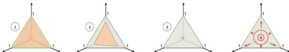
Abundance vectors location corresponding to (1) minimum volume simplex with pure pixels, (2) no pure pixel, (3) all abundances equal to  $\frac{1}{J}$ , and constraint on the dispersion of the abundances
