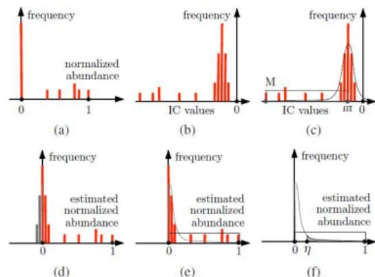
**Fig. 1.** Histogram schemes (a) of a rare endmember abundance map and (b) of the associated IC histogram; (c) scheme of the IC histogram probabilistic model, (d) histogram scheme of the estimated normalized abundance map, (e) scheme of the normalized abundance map probabilistic model and (f) scheme of the threshold computation;
