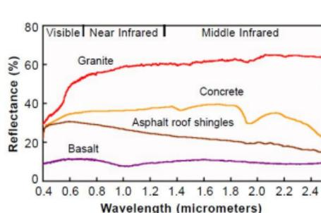
Sample spectra from the ASTER Spectral Library. ASTER will be one of the instruments on the planned EOS AM-1 satellite, and will record image data in 14 channels from the visible through thermal infrared wavelength regions as part of NASA's Earth Science Enterprise program.
