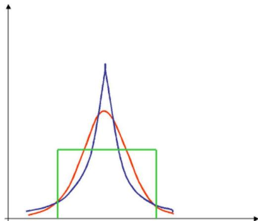
Gaussian, supergaussian (Laplace) and subgaussian (uniform) distributions
