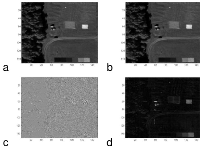
Mean value of original data (a), mean value of reconstructed data with only 5 components (b), direct mean error reconstruction (c) and sqrt of quadratic error reconstruction (d).
