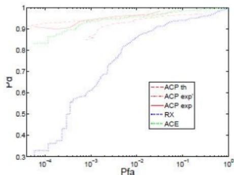
Fig. 3. Detection ROC curves of ACP, ACE and RX. ACP and RX are unsupervised detectors whereas ACE is supervised. These curves have been obtained from the HYDICE dataset presented in Fig.1.
