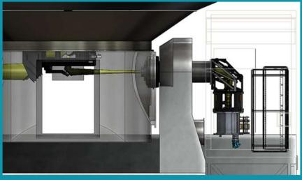
Transmitter of 104 GHz radiation for the Holographic System to be used to adjust the position of the pannels of the antenna dish Mounted by LME group at Escola Politecnica, USP
