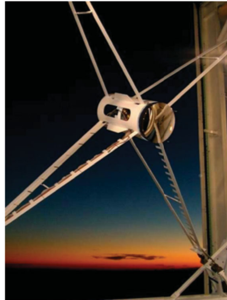
Figure 1. The world's first adaptive secondary: a 65cm 336 actuator ASM at the MMT.
