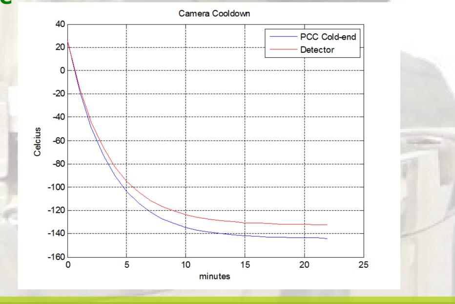
Note that this dynamic simulation does not take into account the thermal inertia of the camera (a time constant), which is assumed to be zero for the simulation. It is only relevant to show the evolution of the two temperatures (PCC and detector) while cooling down.
