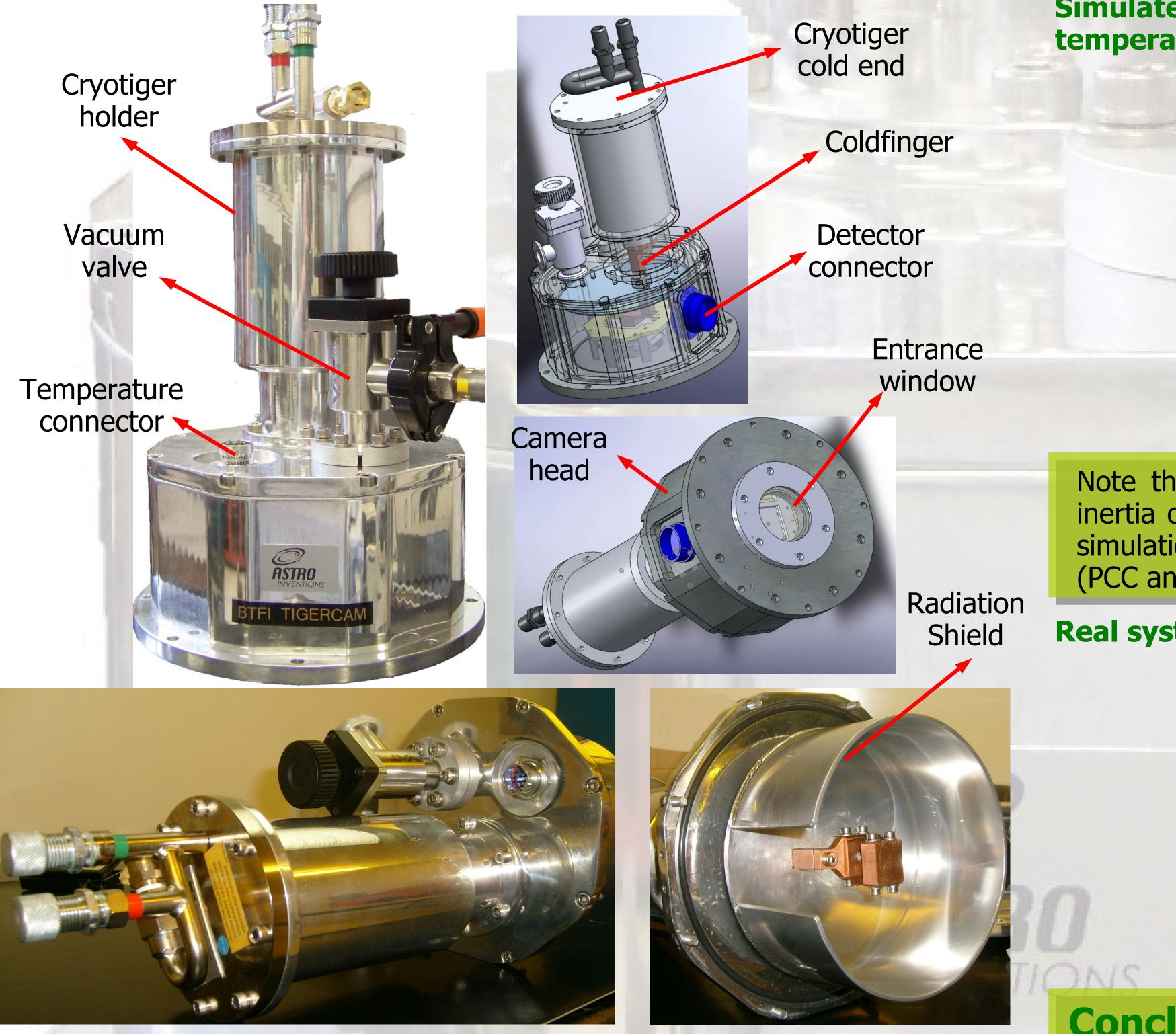
PR<sub>window</sub>: heat transfer by radiation from the camera window;
