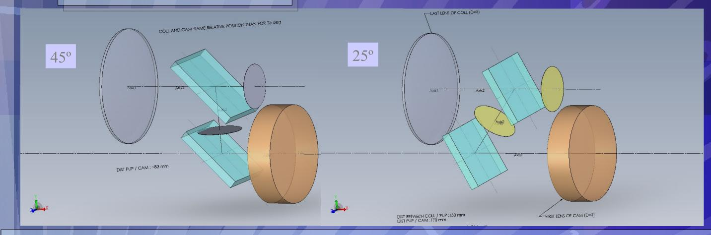
The twin identical VPHGs (blue) following the collimator (grey) such produce dispersion cancellation permitting only the blaze profile to be passed to the camera (gold). The blaze profile is tuned by varying the angle between 45° and 25°. The dispersed and 0<sup>th</sup> order (undeviated) and pupils are shown.
