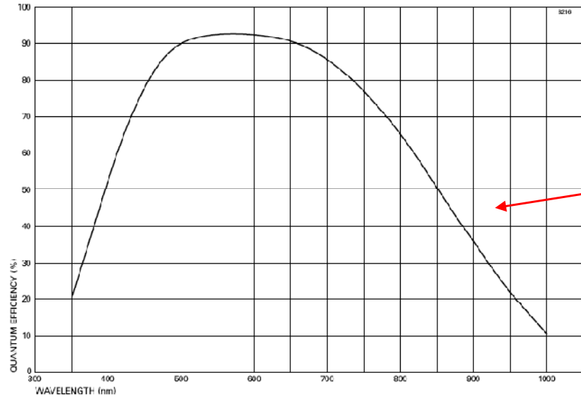
Figure 3: TYPICAL SPECTRAL RESPONSE (At -20^{\circ}\text{C} , no window, midband coating)
