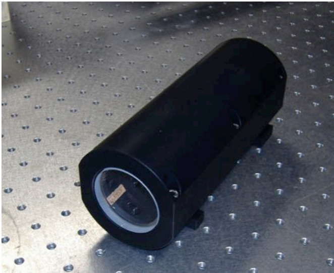
Ammonia gas cell
