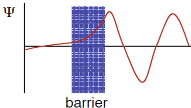
Probability of finding particle  $\sim |\psi|^2$  - if barrier is not too wide then non-zero wavefunction allows some probability of tunnelling...
