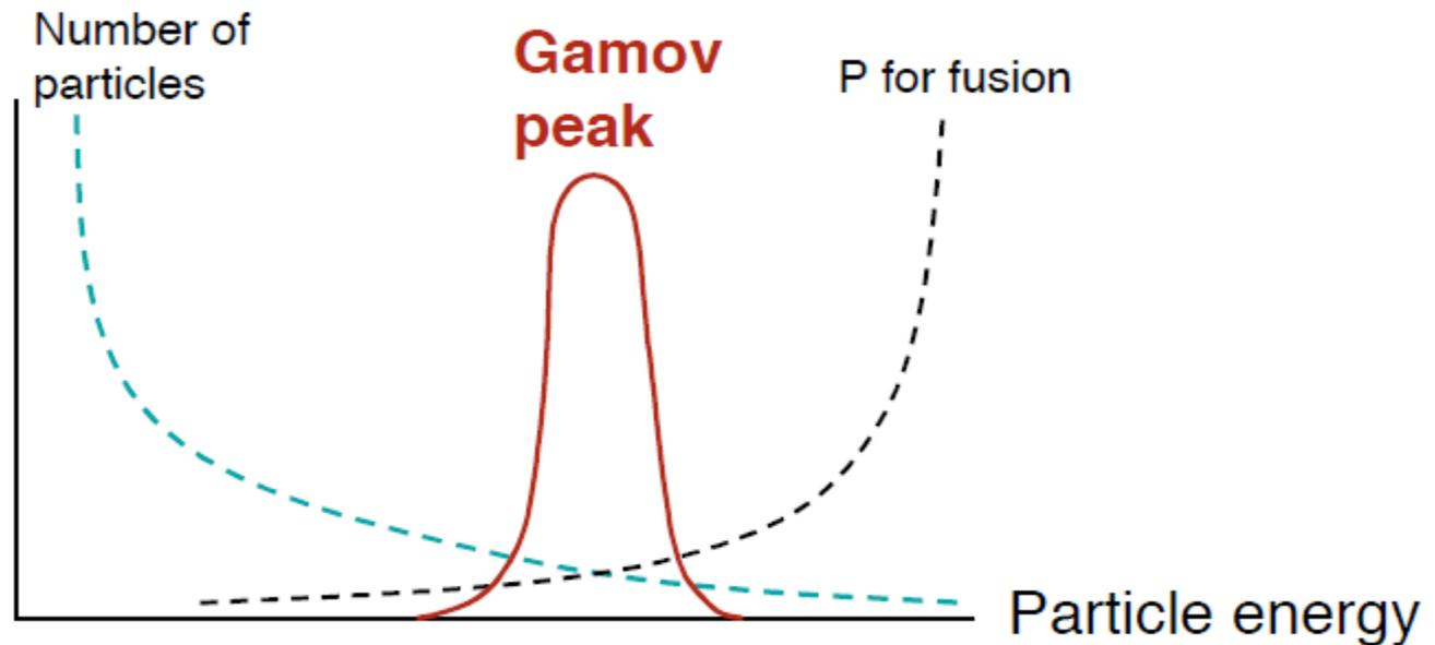
Narrow range of energies around the Gamov peak where significant numbers of particles in the plasma are able to fuse. Energy is  $\gg$  typical thermal energy, so fusion is slow.
