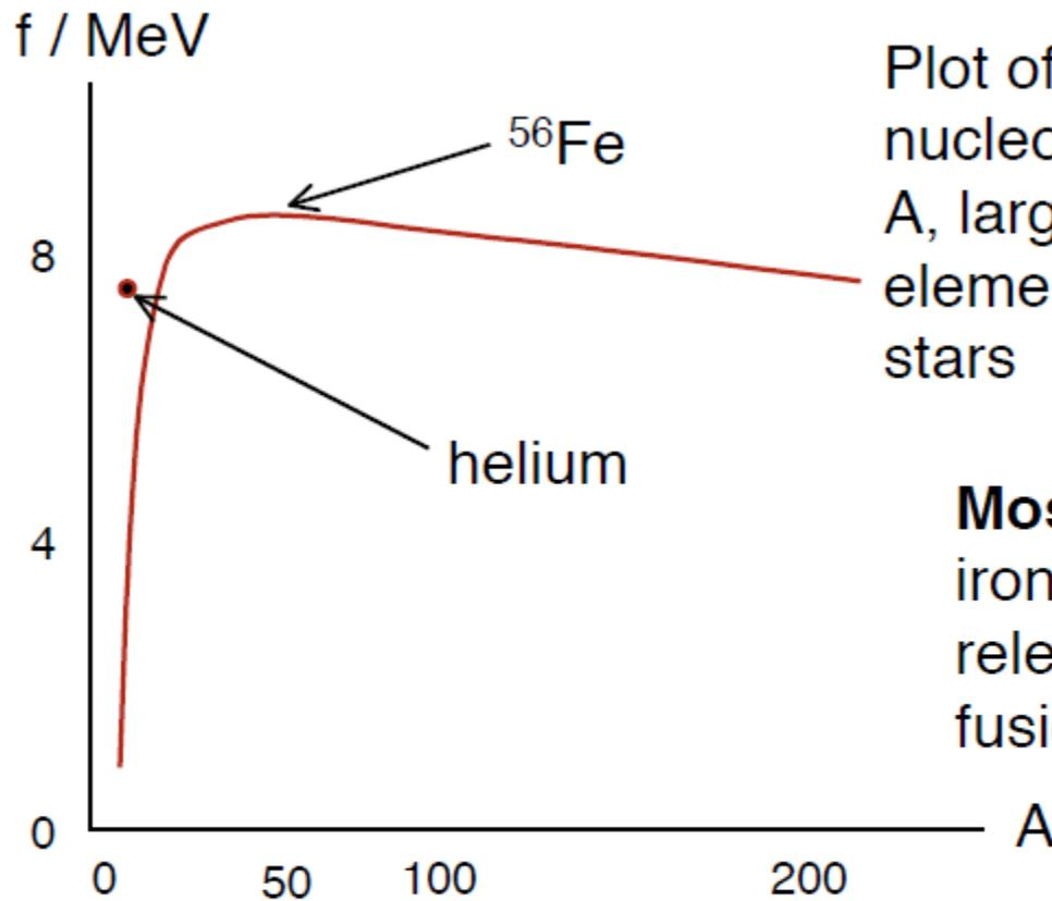
Plot of binding energy per nucleon,  $f$ , vs. atomic number  $A$ , largely determines which elements can be formed in stars
