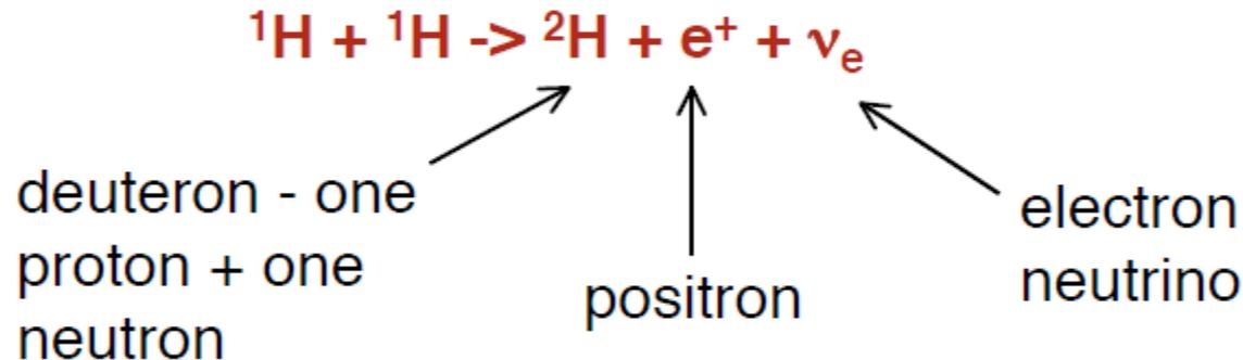
This is the critical reaction in the proton-proton chain. It is slow because forming a deuteron from two protons requires transforming a proton into a neutron - this involves the weak nuclear force so it is slow...
